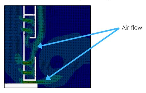
Side view of top trim. Air flows through holes in trim from inside refrigerator cabinet into room.
