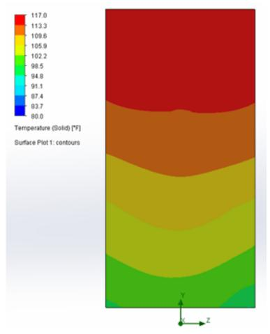
Plot of temperature at back of refrigerator with trim kit installed and operating in 80° F room. Temperature is highest near the top of the refrigerator.
