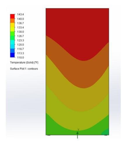
Plot of temperature at back of refrigerator. Temperature is highest near the top of the refrigerator.
